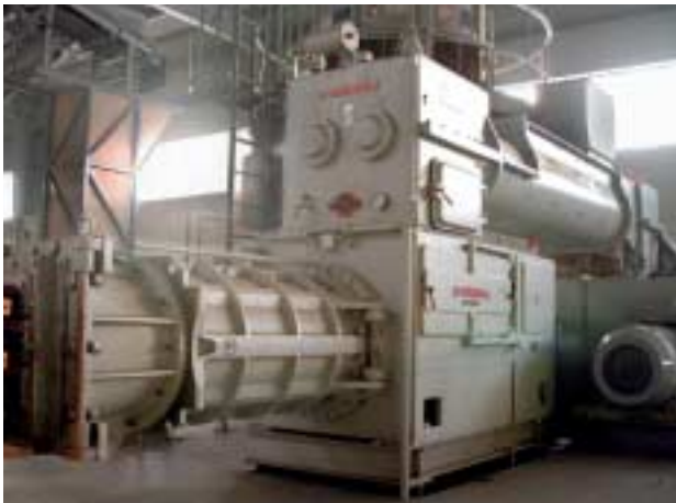
»8 Futura-Vakuumaggregat »8 Futura combined de-airing extrusion unit
