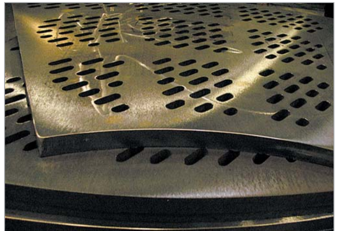
Grid/ screen-plate perforations to fit the respective degree of conditioning, delivery rate and wear pattern
