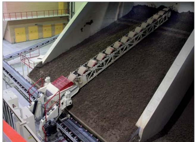
Efficient system for storing and retrieving raw materials: HÄNDLE's new longitudinal-dredging excavator program
