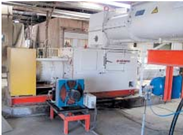
»12 Futura combined de-airing extrusion machine, mixer installed transversely to the extruder
