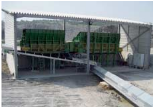
»3 Box feeder station in the pit – the open air stockpiles seen in the background with the belt conveying system for material transport to the factory in front »3 Beschickerstation in der Grube – in der Kulisse die Freihalden, davor die Bandstraße zum Werk
