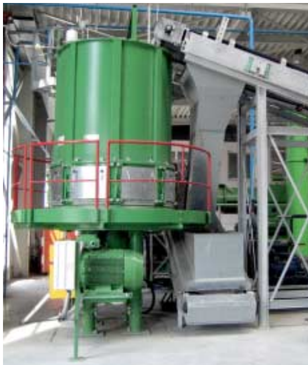
»12 Clay shredder model BRSH 19b with screen cover to prevent material from drying out, with by-pass system via chute and reversible belt conveyor
