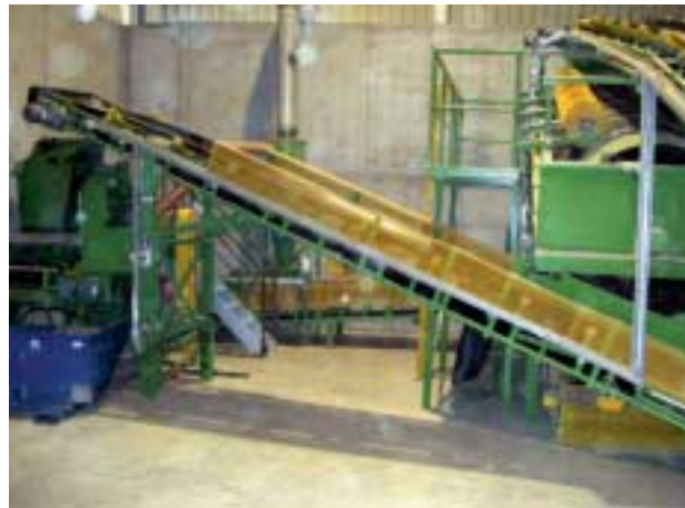
»9 Saw dust preparation – rotary screen on the right (with cleaning brush to remove sticking wood fibres), on the left saw dust grinder (with incorporated screen, in the foreground the container with eliminated coarse matter)
